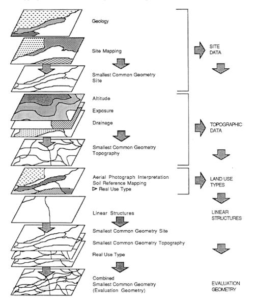
Figure 4. The process of sieve mapping
