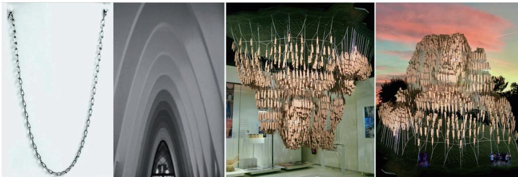
Figure 12. Left: catenary (free-hanging chain) and parabolic-catenary arches. Right: a string model, hanging from the ceiling with bags of sand to calculate the weight proportional to that of the real construction
