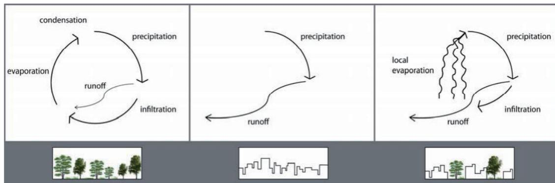
Figure 1: Water cycle in different phases a) in natural system (left); b) in urban area without sustainable storm water management (middle); c) in an urban area with sustainable storm water management (right)
