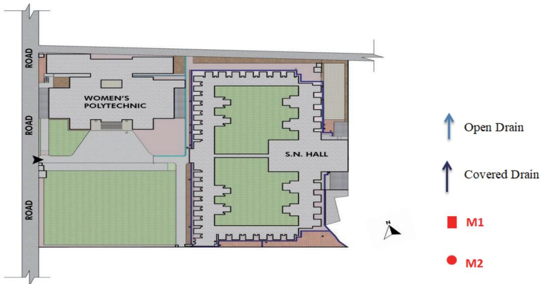
Figure 9: The drain layout of existing condition
