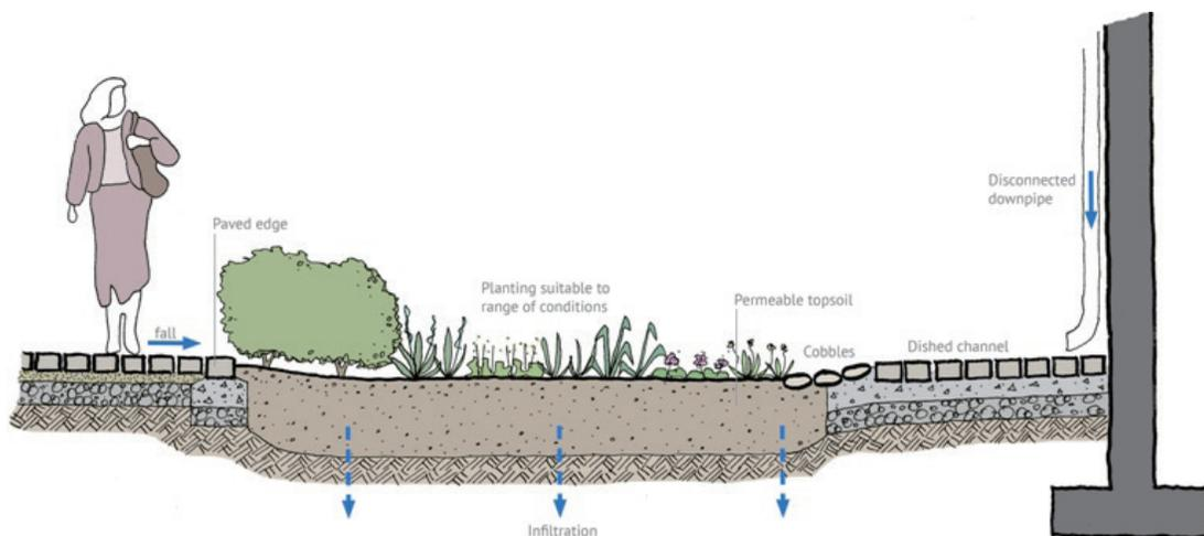
Figure 4: The details of infiltration trench
