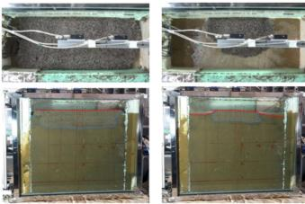
(c) After 0.2g vibration (d) After 0.3g vibration Figure 1. The macroscopic phenomena on liquefaction of sand
