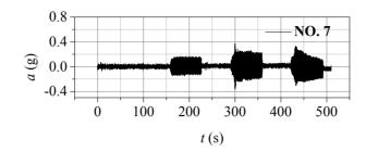
Figure 3. Acceleration history curves of different monitoring points
