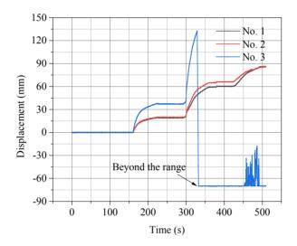
Figure 2. Settlement history curves of different monitoring points
