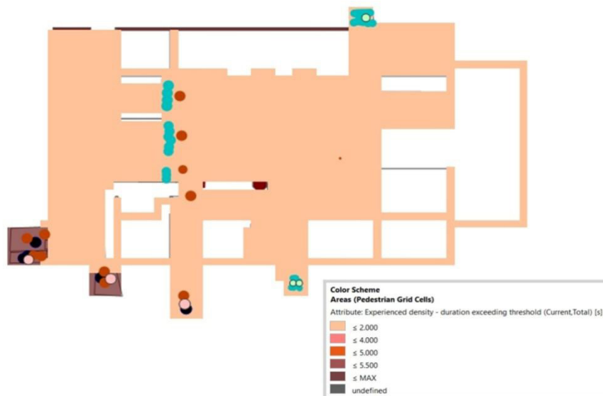
Figure 9. Experience Density map exceeding Threshold (Total) for 1 hr simulation run.
