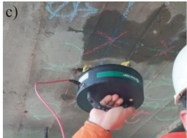
Figure 9. a) Definitions of serviceability level (performance) of a structure over time (ISO16311, 2014), b) NDT measurements of carbonation and chloride ingress and c) level of reinforcement corrosion.
