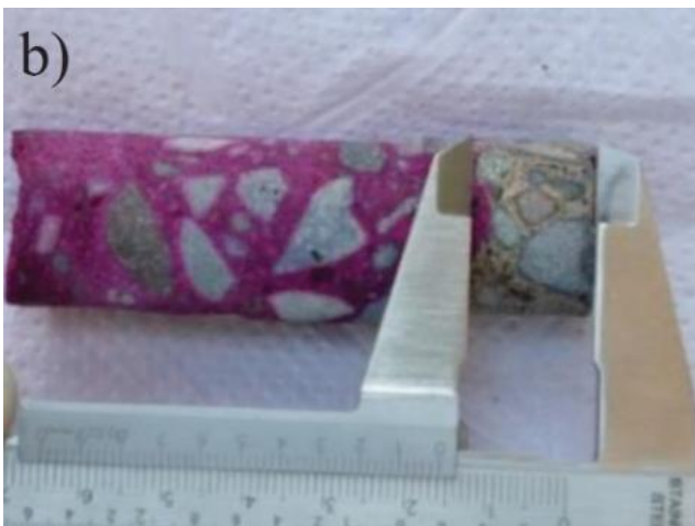
Figure 9. a) Definitions of serviceability level (performance) of a structure over time (ISO16311, 2014), b) NDT measurements of carbonation and chloride ingress and c) level of reinforcement corrosion.
