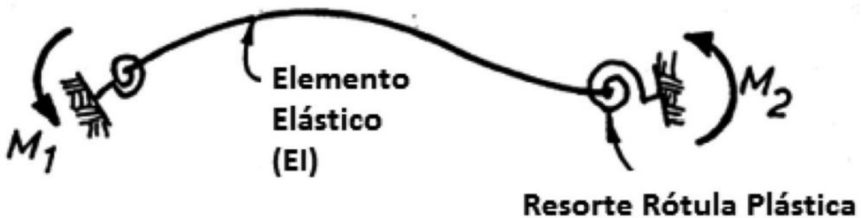
Figure 10. Giberson-type element for modeling nonlinearity in original structure without hybrid junctions.
