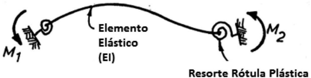
Figure 10. Giberson-type element for modeling nonlinearity in original structure without hybrid junctions.
