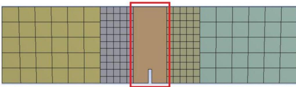
**Figure 4.** Finite element meshing of notched beams.
