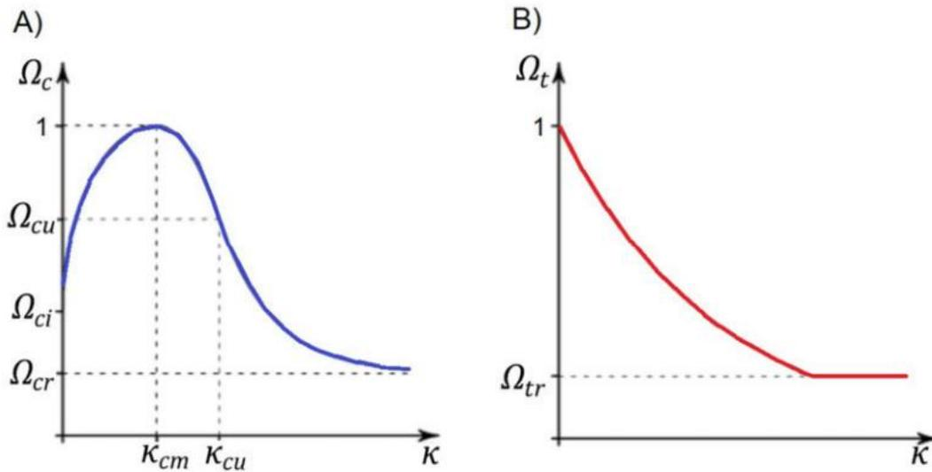
**Figure 2.** Hardening and softening functions in (A) tension and (B) compression.
