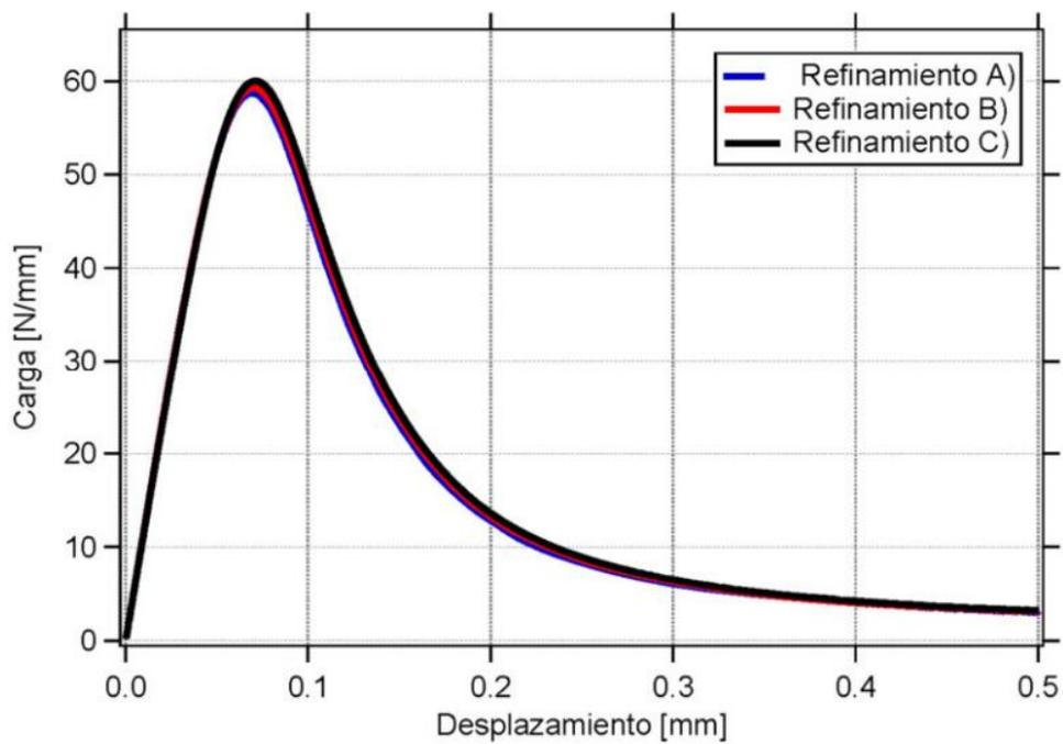
**Figure 6.** Load-displacement curves. Effect of mesh size.
