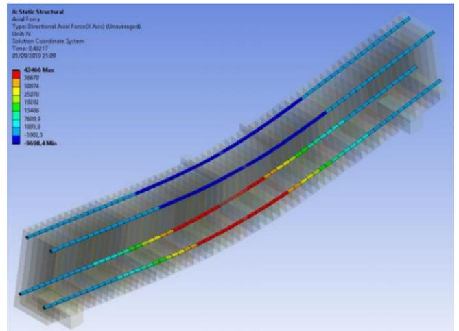
Figure 17. Deformation of the bars of Test 3 for a displacement of 5 mm. Deformation x50.
