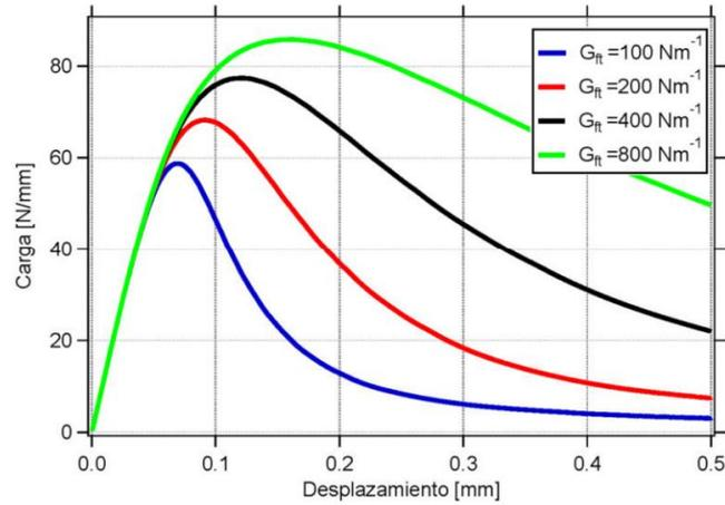
**Figure 7.** Load-displacement curves. Effect of fracture energy.
