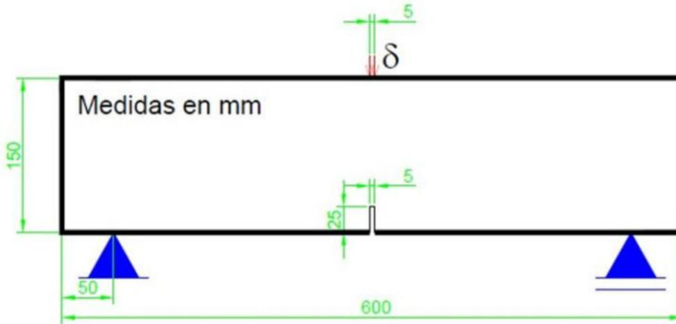
**Figure 3.** Schematic diagram of notched beam bending tests.
