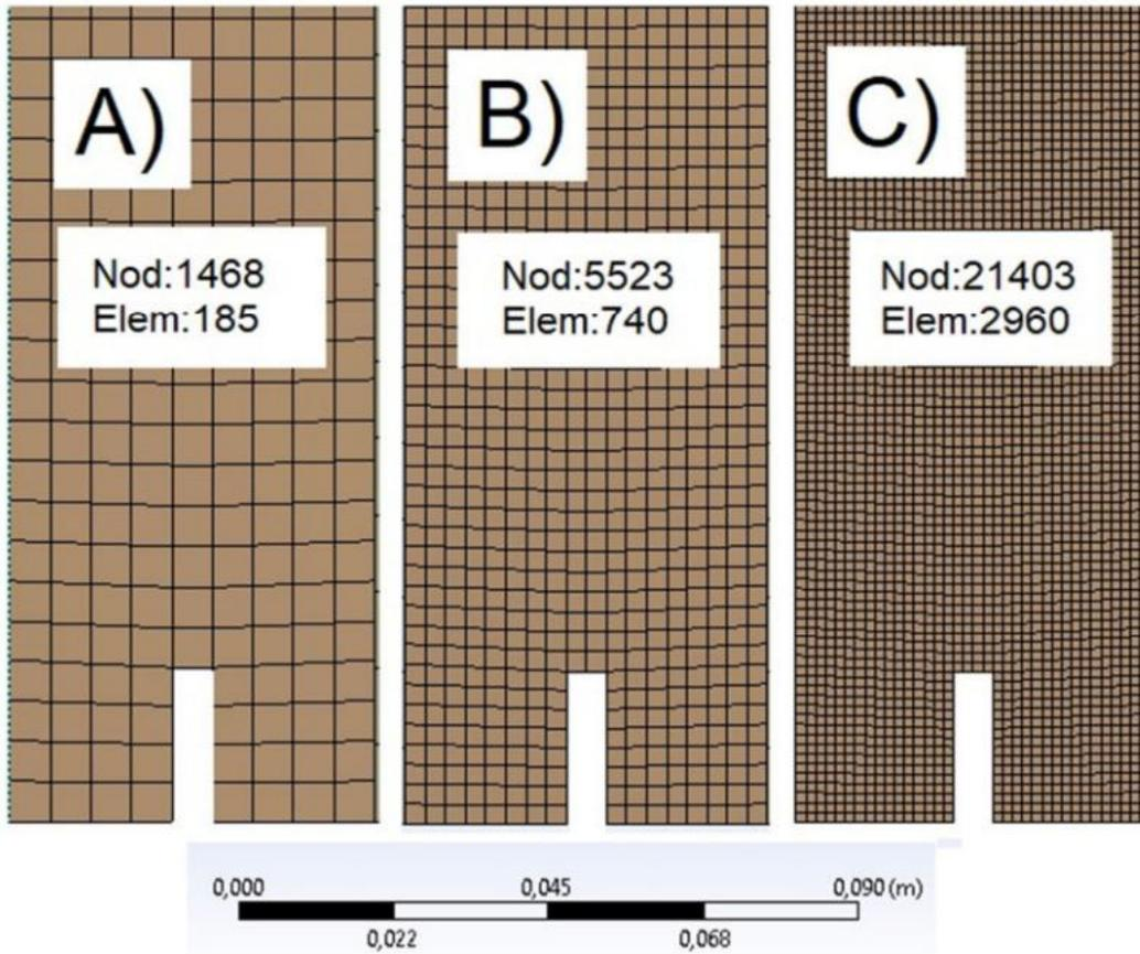
**Figure 5.** Mesh refinements in the center section of the notched beams.
