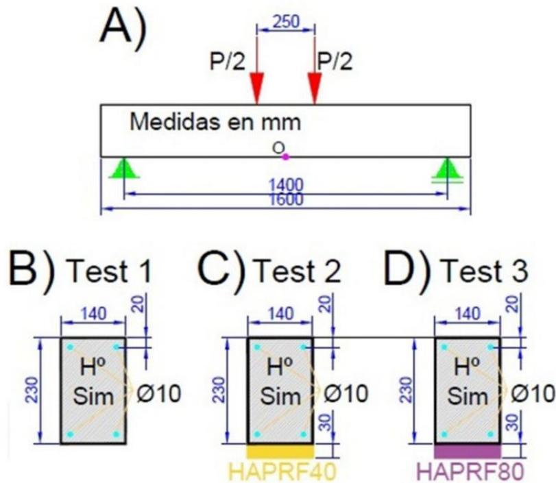
**Figure 12.** Tests of H° beams reinforced with HPFRC.
