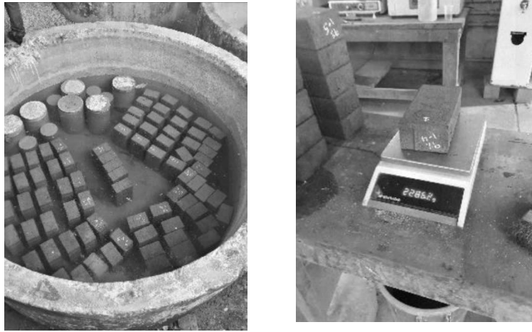
Figure 5. 24-hour saturation and weighing of paving stones
