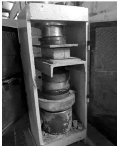
Figure 10. Setup for 28-day compression test
