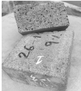
Figure 8. Pathological result of paving stone flexural failure
