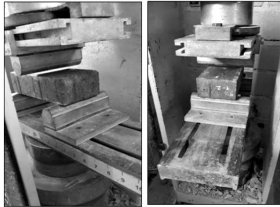
Figure 7. Setup for 28-day flexural tensile test
