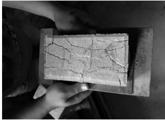
Figure 11. Pathological result of compressive failure of the paving stone
