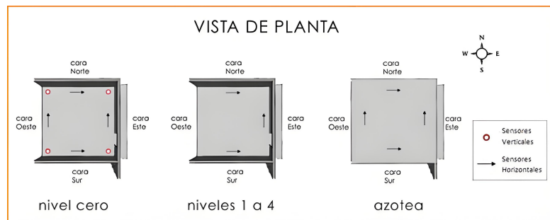
Figure 9. Location of the vertical and horizontal sensors in the experimental building.
