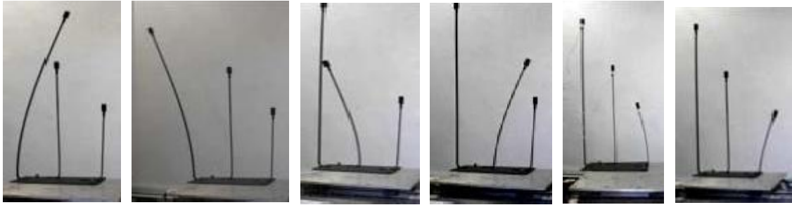
Figure 5. Resonance of each pendulum for different soil vibration periods
