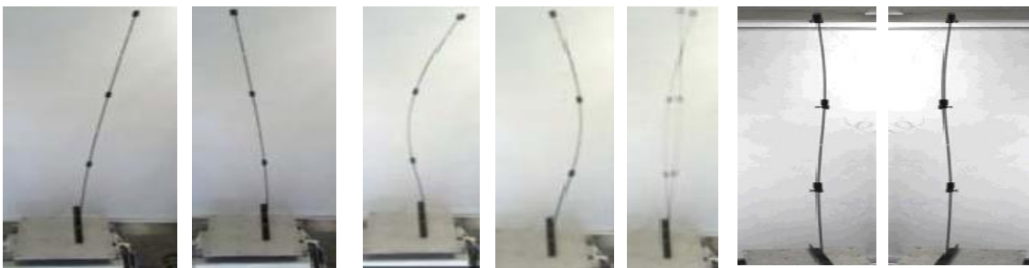
Figure 7. Three-mass pendulum vibration modes
