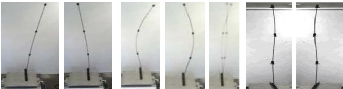
Figure 7. Three-mass pendulum vibration modes
