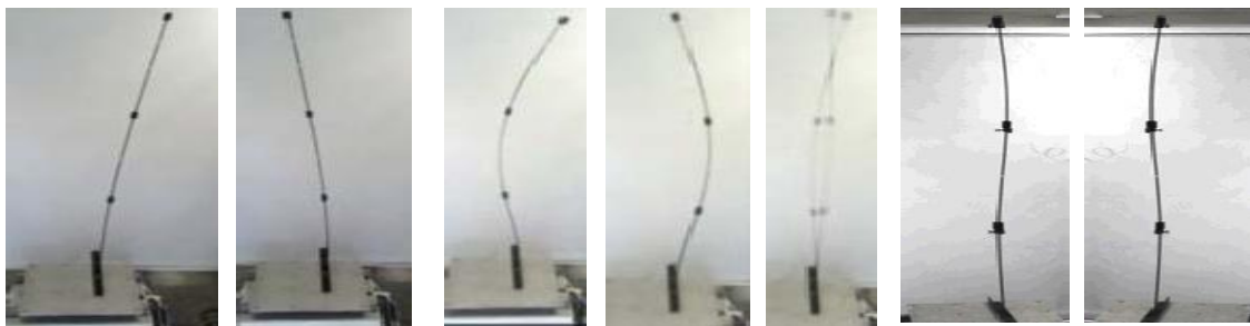
Figure 7. Three-mass pendulum vibration modes
