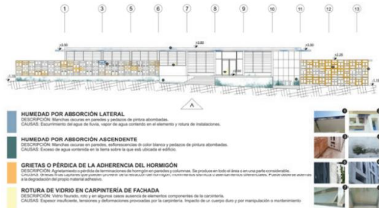
Figure 6. Damage report for elevation A. Source: authors, 2023
