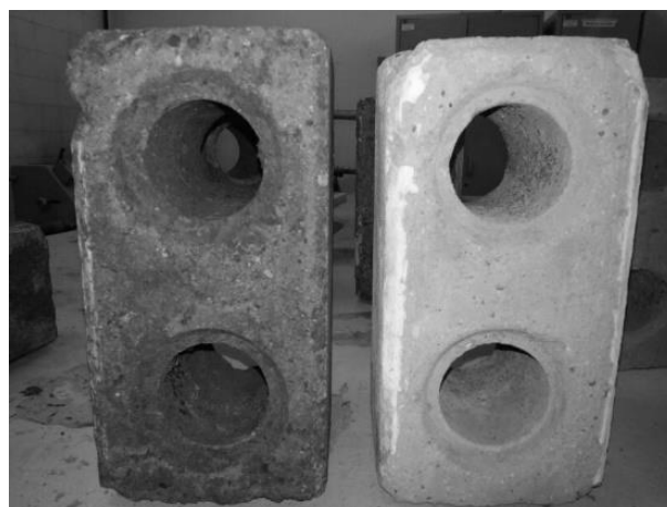
Figure 1: Image of soil-cement block samples taken from the construction site. Source: the author
