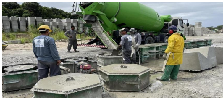
Figure 4. Manufacturing of the hexagonal rings. Source: the authors
