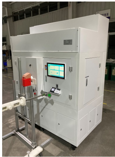
Figure 4. Field test of radiated RF electromagnetic field immunity test for a sampling robot
