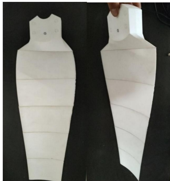
Figure 24. 3D printed manufacturing blade model, scale 1:1 Source: Own elaboration
