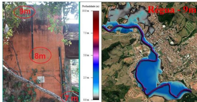
Figure 14. Photo of the limnometric ruler with the flood stain at a height of 9 m
