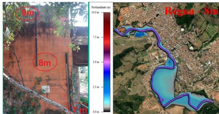
Figure 13. Photo of the limnometric ruler with the flood stain at a height of 8 m
