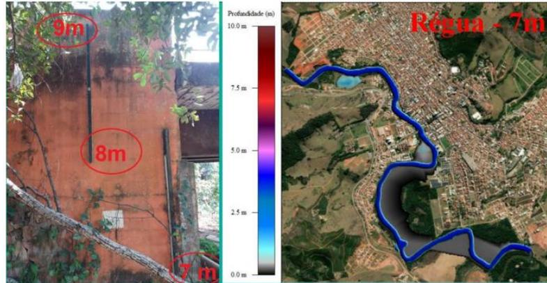
Figure 12. Photo of the limnometric ruler with the flood stain at a height of 7 m
