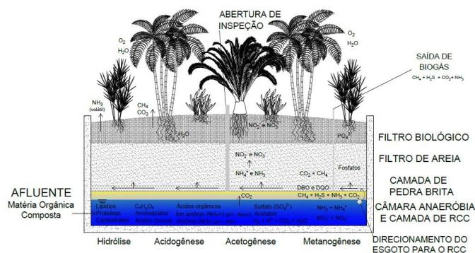
Figure 1. TEvap operation diagram
