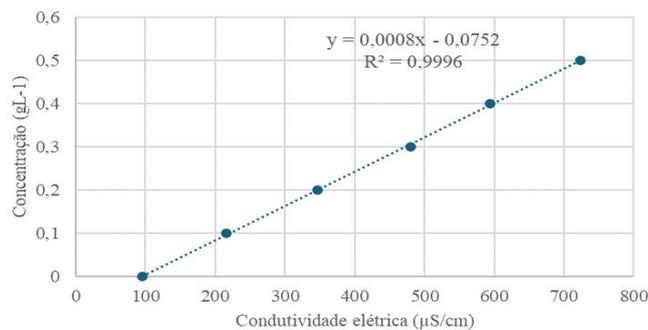
Figure 3. NaCl concentration curve by electrical conductivity
