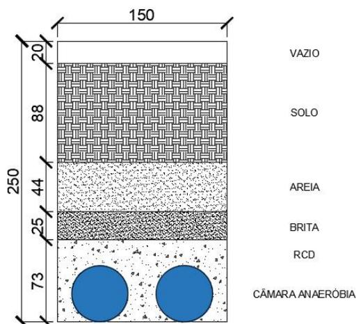
Figure 2. Layers that made up the experimental apparatus
