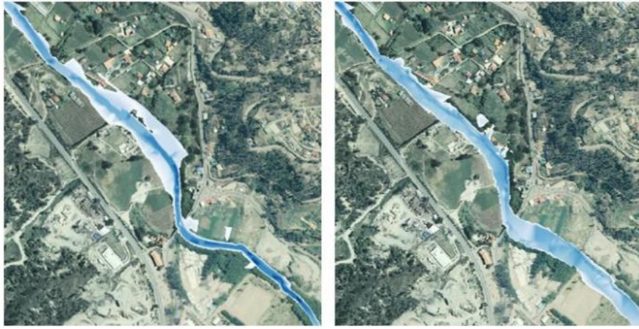
Figure 18. On the left, flood patch with scenario one and on the right, flood patch with scenario two, for a 100-year return period
