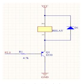
Figure 3. Relay circuit
