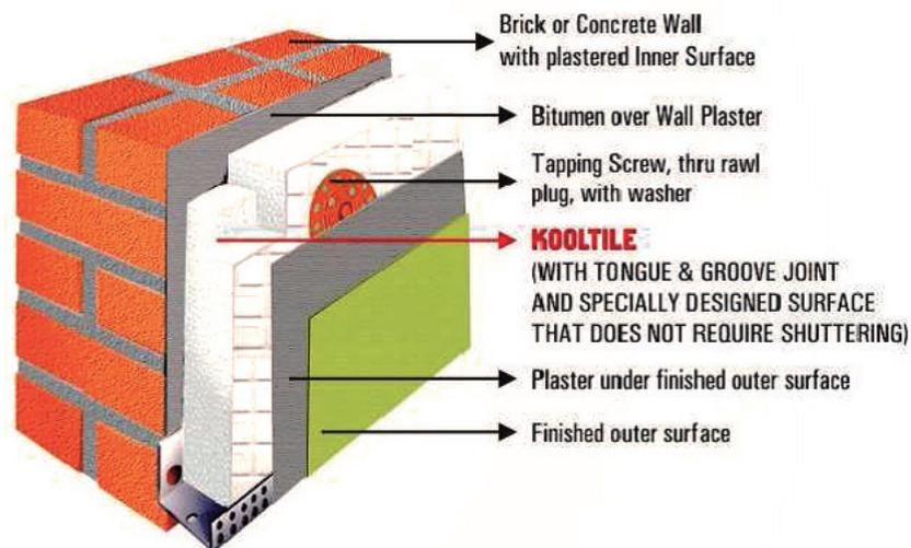
Figure 15. Section showing the procedure of installing insulated EPS tiles on the wall surface
