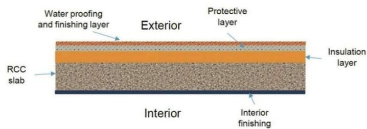
Figure 4. Details of roof insulation above the floor slab
