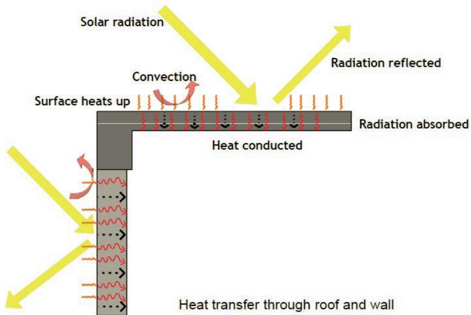
Figure 2. Exposure of solar radiation on the building envelope and thermal heat conduction
