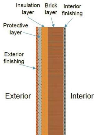
Figure 6. Wall with external insulation
