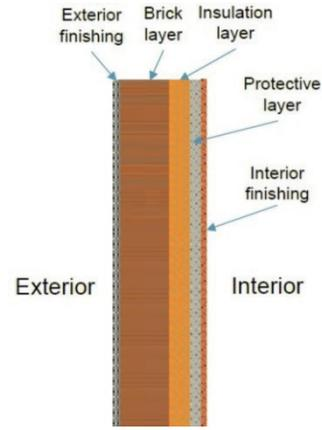
Figure 7. Wall with internal insulation
