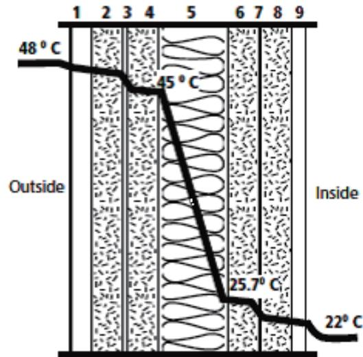
Figure 9. A Section of an insulated EPS Tile
