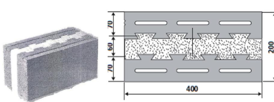
Figure 8. View of a block and a sectional plan of a Kool Tile
