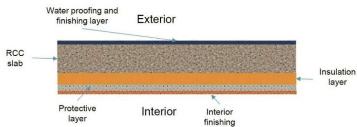
Figure 5. Details of roof insulation below the floor slab
