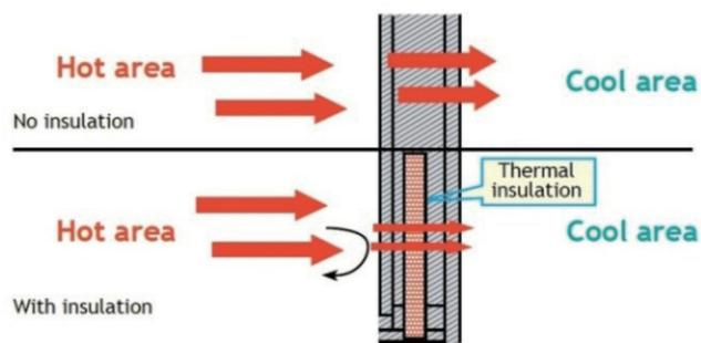
Figure 3. Effect of thermal insulation on heat transfer through walls
