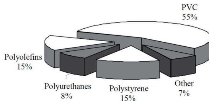
Figure 1. Plastics in building and construction
