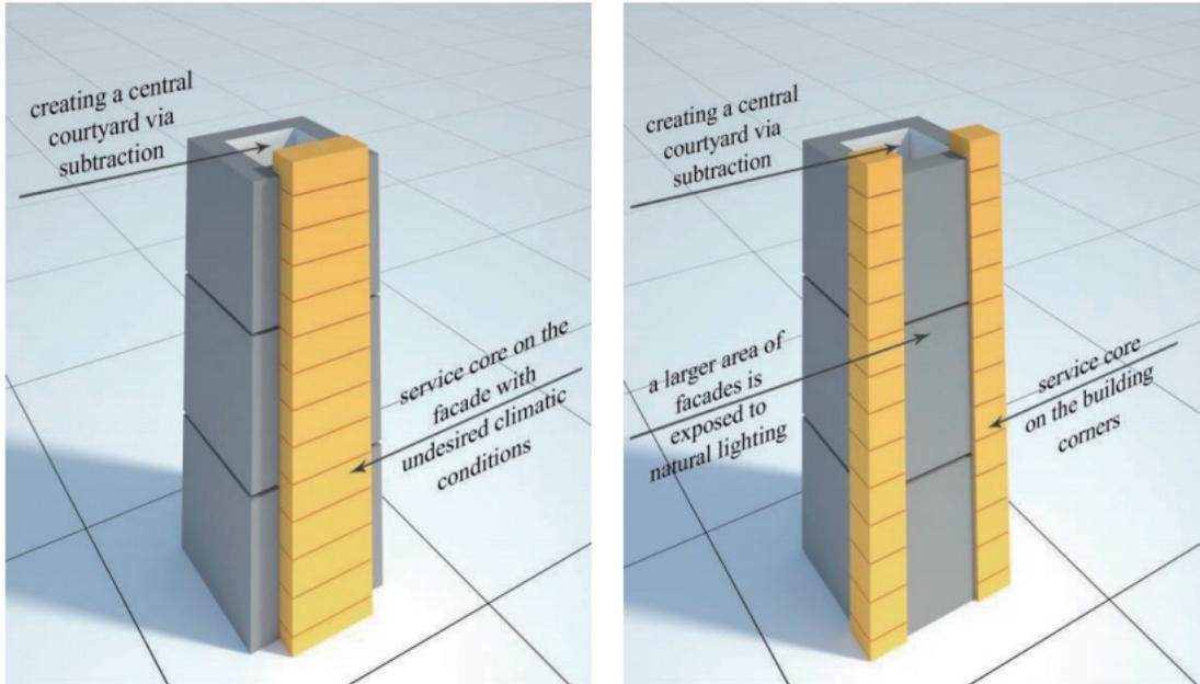
Figure 5. The location of service core in a high rise building
