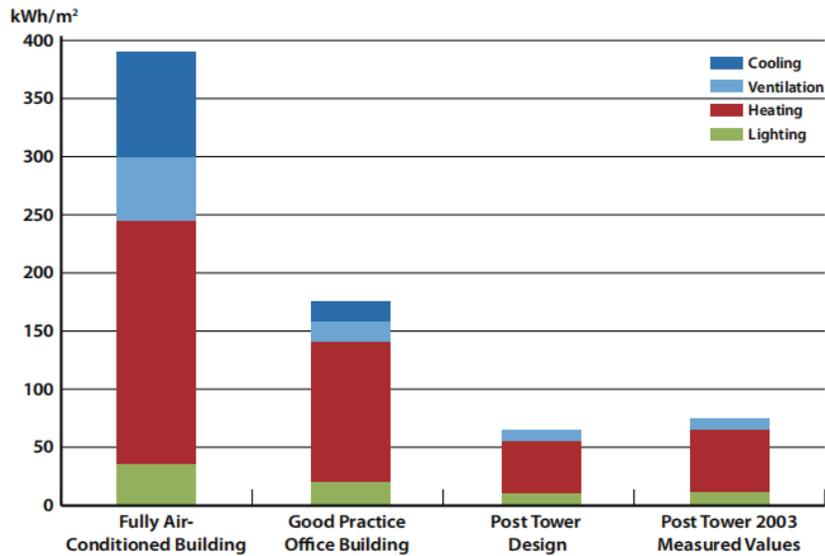
Figure 18. The energy performance of the Post Tower
