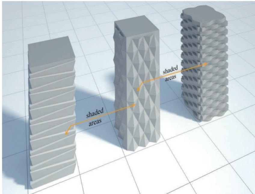
Figure 7. The impact of pattern on the building facade
