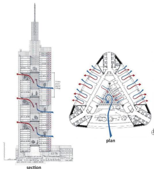
Figure 10. The plan and section of Commerzbank at Frankfurt, Germany
