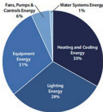
Figure 3. Average Energy consumption in a typical rise-rise office building
