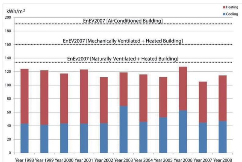
Figure 13. Annually energy consumption for heating and cooling
