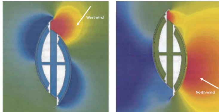
Figure 16. Computational fluid dynamic studies showing the effect of wing walls
