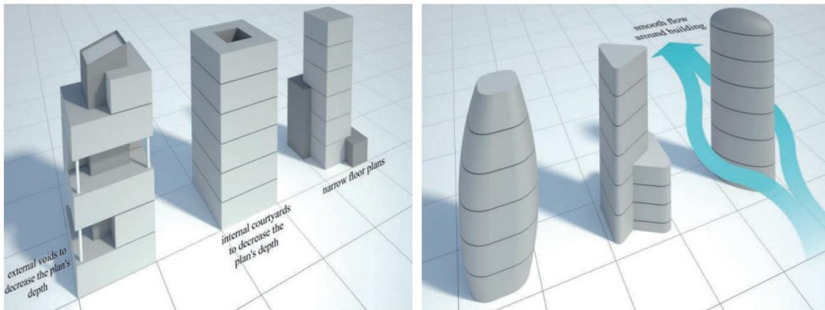
Figure 6. The impact of building shapes and aerodynamic form on energy consumption
