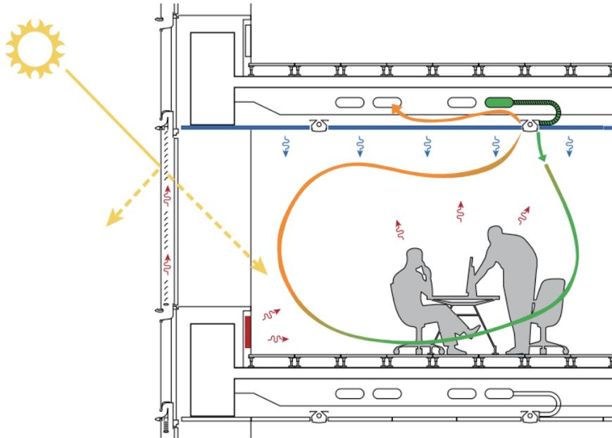
Figure 14. The HVAC system in the building both in winter and summer
