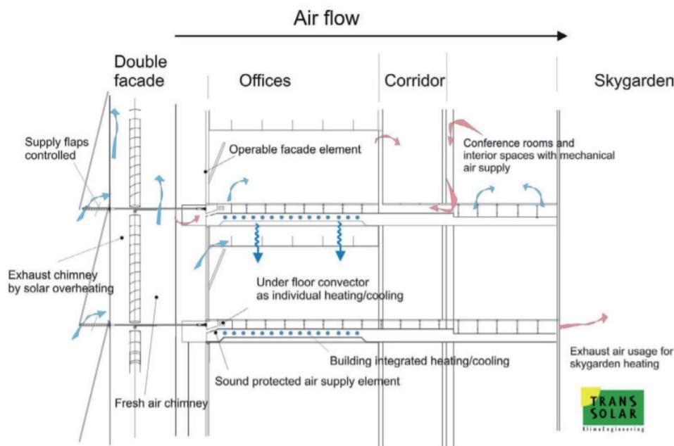
Figure 19. Sectional detail of the HVAC system of the Post Tower
