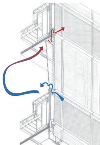
Figure 12. Double-glazed hinged window allows cool air from the cavity to flow inside
