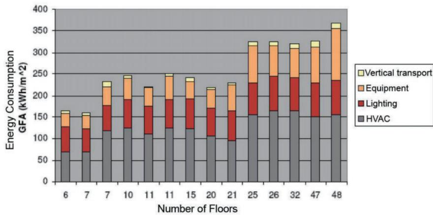
Figure 1. Energy consumption with a number of floors
