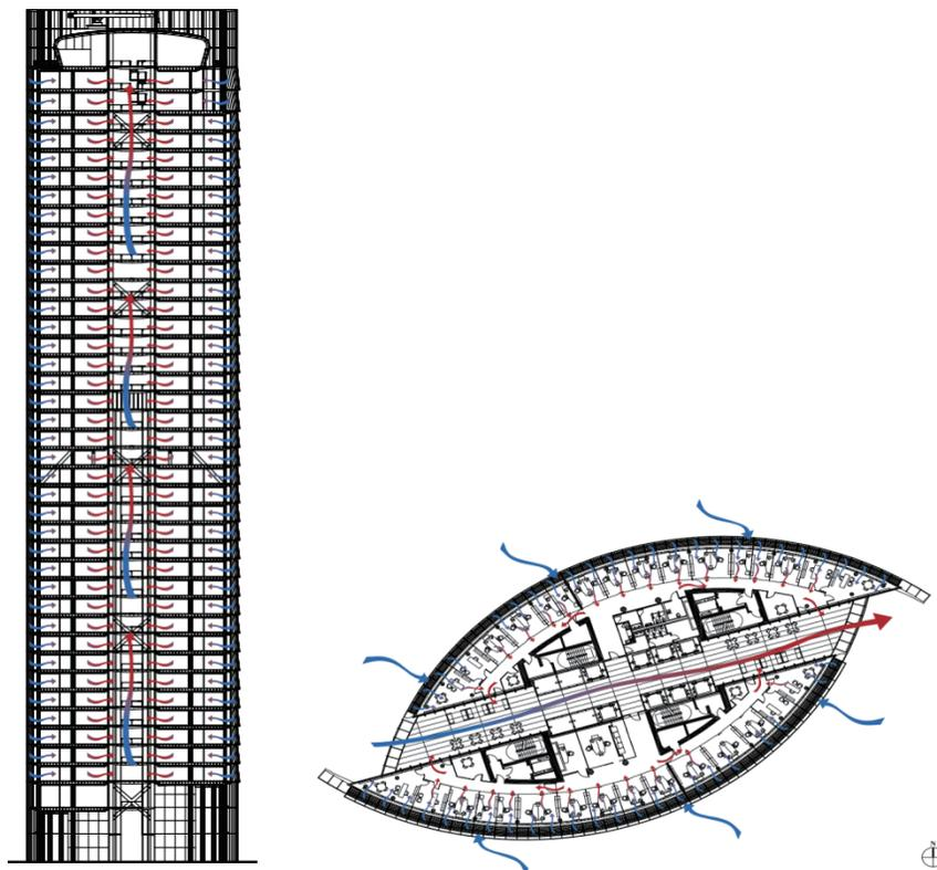
Figure 17. Plan and section showing cross ventilation and stack effect through the sky garden
