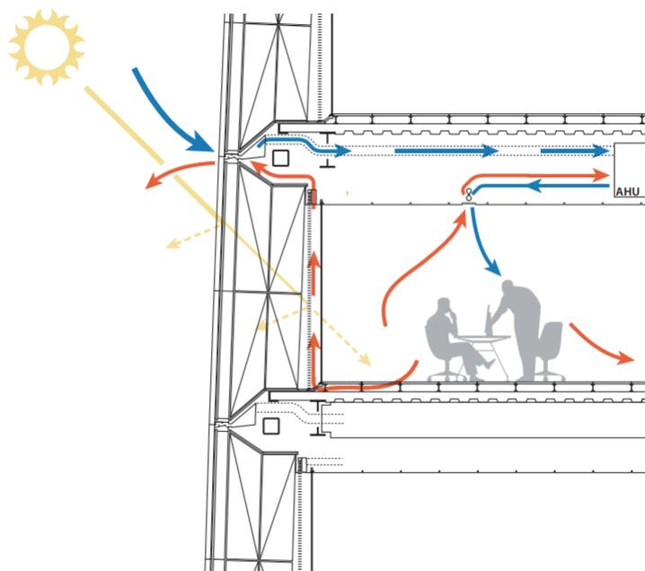
Figure 23. The HVAC system of 30 St Mary Axe
