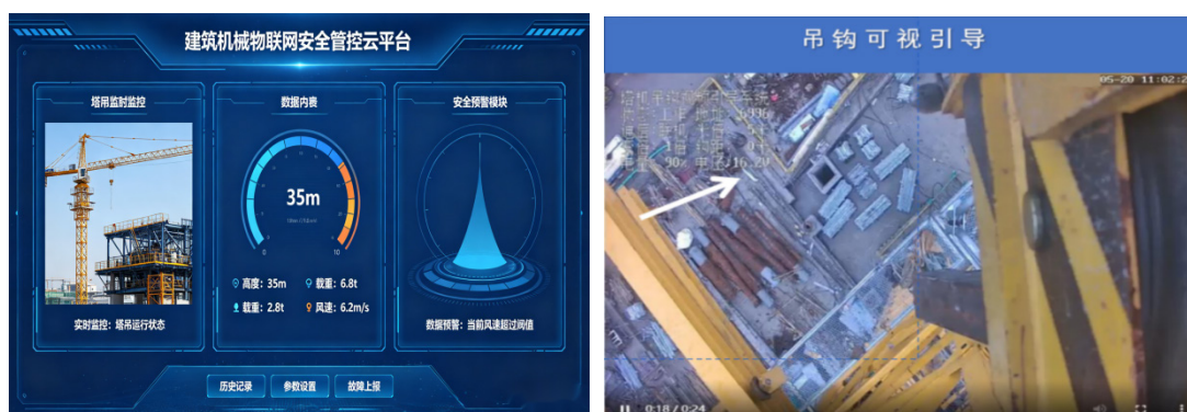
Figure 1. Schematic diagram of the lifting visualization remote platform
