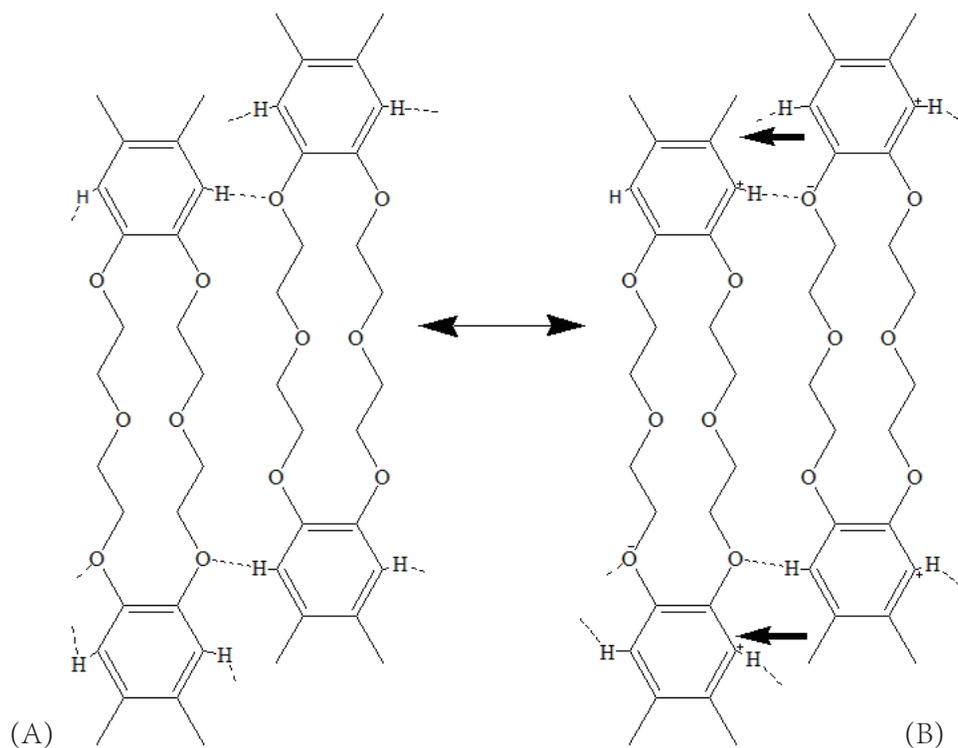
Figure 4. Schematic diagram of PDBC-18 chains which exhibit (A) interconnection through H bonds and (B) charge transfer process to create dipole in a specific direction.
