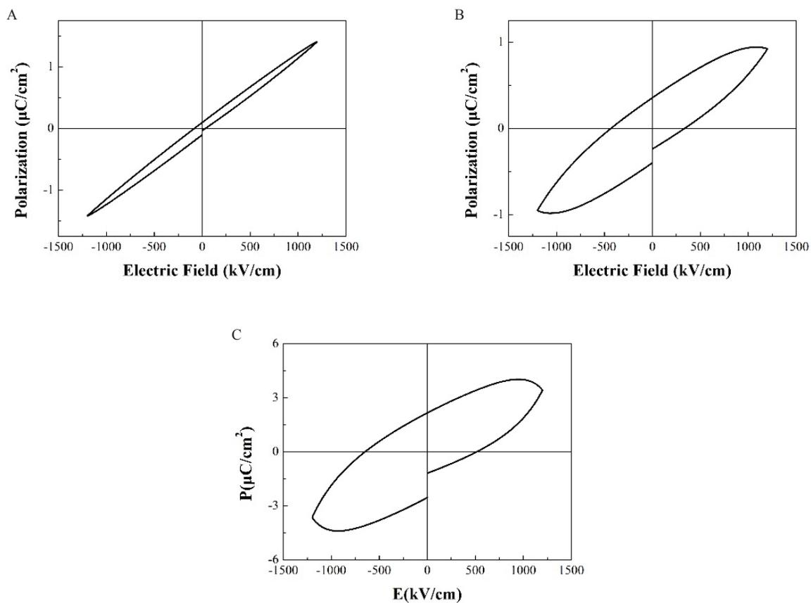
Figure 3. P-E loop at room temperature for (A) PDBC-14, (B) PDBC-15 and (C) PDBC-18. The values of remnant polarization are about 0.1, 0.36 and 2.16  $\mu\text{C cm}^{-2}$ , respectively.
