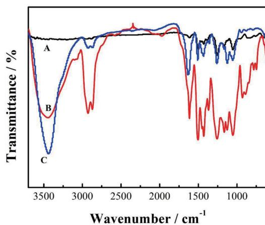
**Figure 2. FTIR spectra of the (A) PDBC-14, (B) PDBC-15 and (C) PDBC-18 obtained potentiostatically at 0.7V, 0.85V and 1.05V, respectively from BFEE + 0.01 mol L<sup>-1</sup> DBC.**
