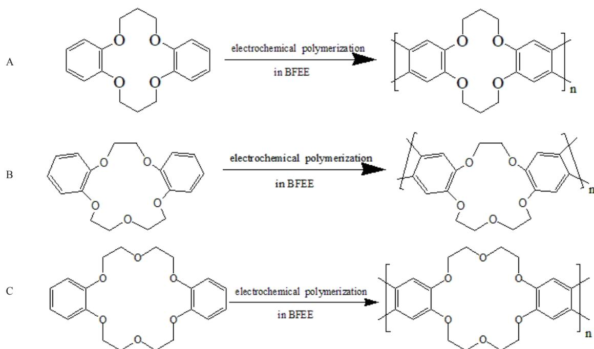
**Figure 1. The electrochemical polymerization of (A) dibenzo-14-crown-4, (B) dibenzo-15-crown-5 and (C) dibenzo-18-crown-6.**
