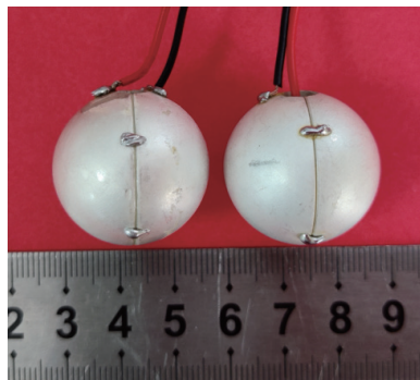
Figure 2. Piezoelectric ceramic ball sample (Sintered spherical shell sample on the left; glued spherical shell sample on the right)
