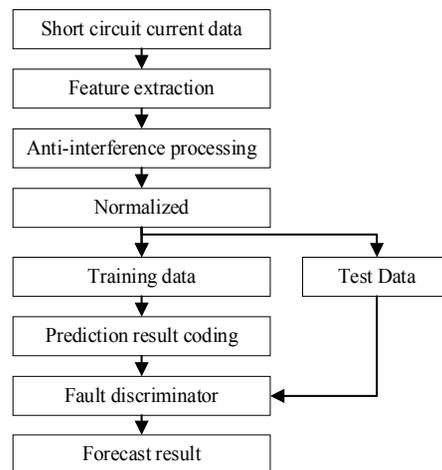
Figure 4. Track circuit fault diagnosis process
