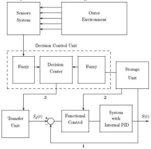
**Figure 6c**. Intelligent Control Structure at Block 3 of **Figure 1** with Decision Centre (here with Fuzzy type Reasoning) Transferring Order To System (Link 3),
