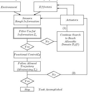
Figure 3. Structure of Filtering Block of Figure 2 with Task Oriented Control
