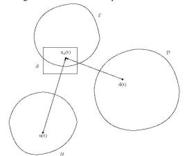
**Figure 7.** Generating Scheme of Solution  $x_s(t, x_s(0), u(t), d(t))$ from Knowledge of Control Functions  $u(t) \in U$  and Disturbances  $d(t) \in D$ . Determination of Subspaces  $D' \subseteq D$ , U' $\subseteq U$  so that  $x_s(t) \in S$  is Done by Application of Fixed Point Theorem in Adequate Function Spaces
