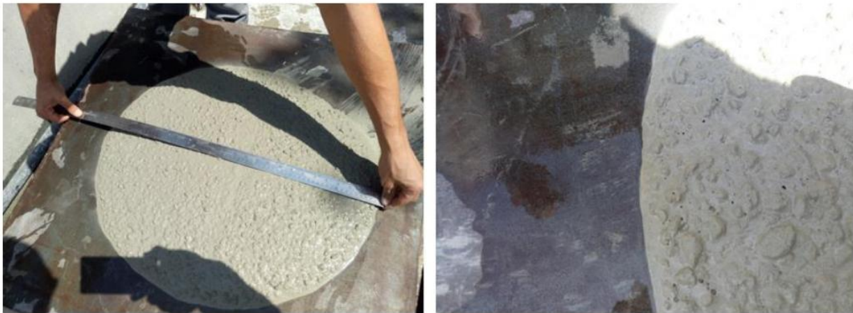
Figure 3. Details of the dispersion test performed in the laboratory during the dosing study.
