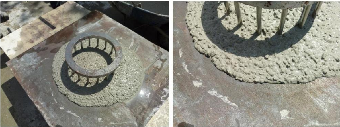
Figure 5. Details of the ability test to pass the J-ring conducted in the laboratory during the dosing study.
