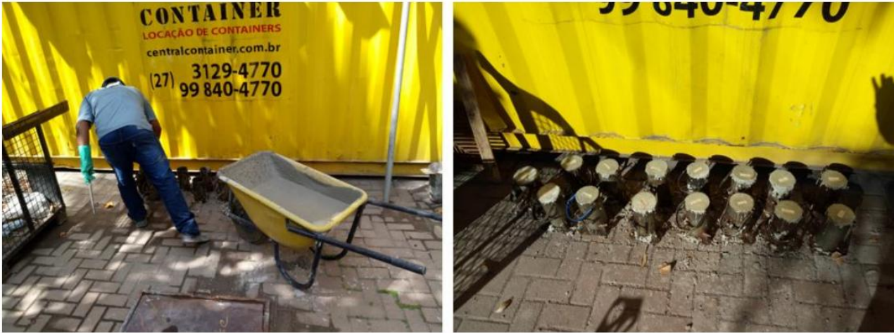
Figure 6. Detail of the cylindrical specimen molds in the prototype casting for compressive strength tests and modulus of elasticity tests.
