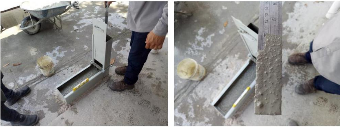
Figure 4. Details of the ability test to pass the L-box conducted in the laboratory during the dosing study.
