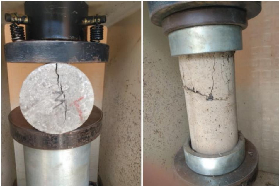
Figure 6. Tensile and compressive strength tests. Source: Own elaboration.
