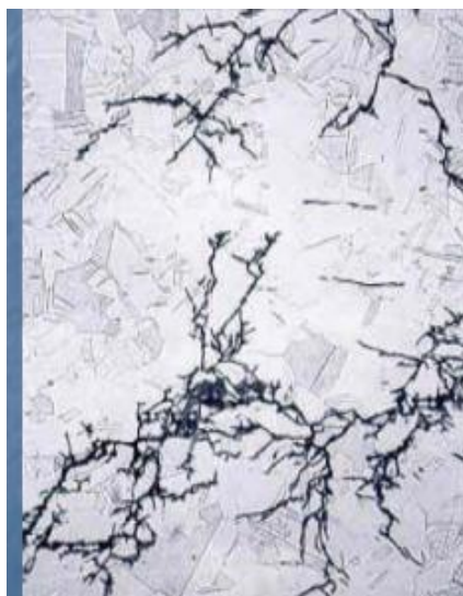
Figure 9. Under stress corrosion.
