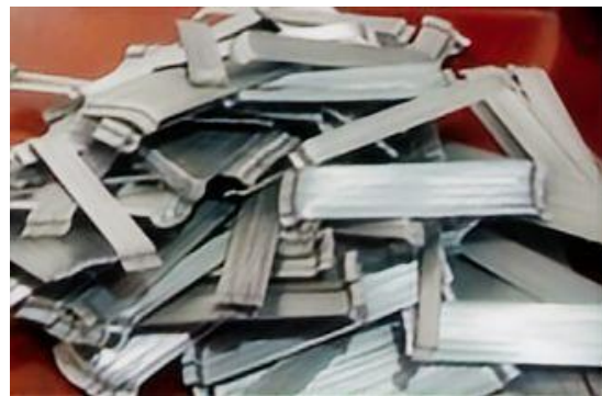
Steel fibers with hooks at the ends
