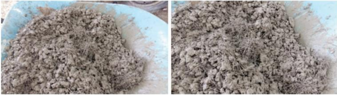
Figure 5. Concrete mix with synthetic corrugated fibers.
