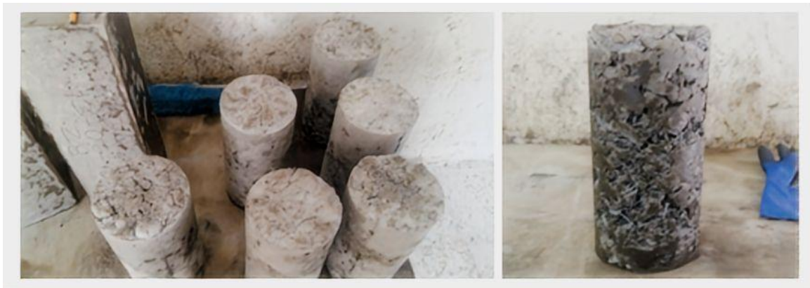
Figure 4. Concrete specimens reinforced with 1.00% and 1.50% fibers.
