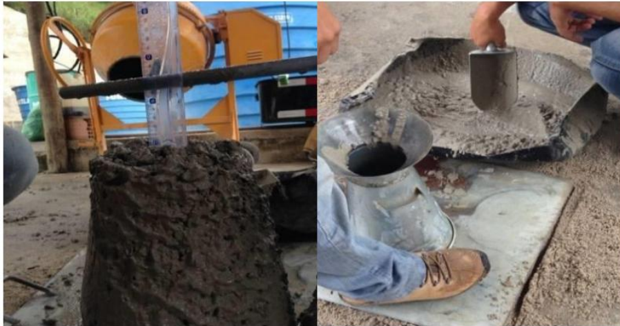
Figure 1. Slump test. (Source: Author's personal archive)
