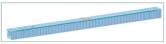
Figure 6. Medium plate finite element model
