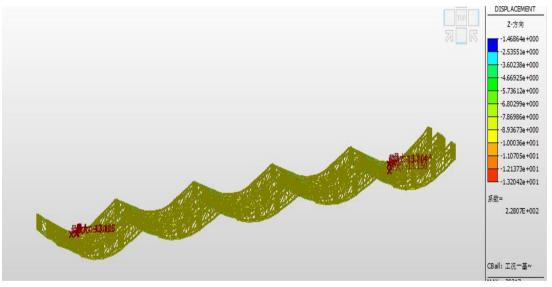
Figure 6-6. Check deflection diagram of Bailey beam (unit: mm)
