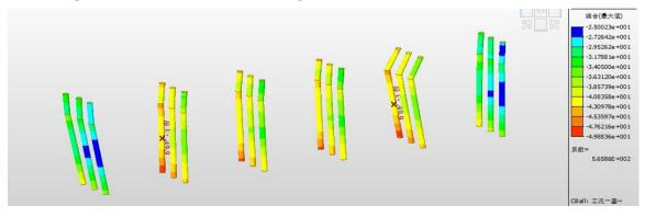
Figure 6-9. Stress calculation diagram of steel pipe pile (unit: MPa)
