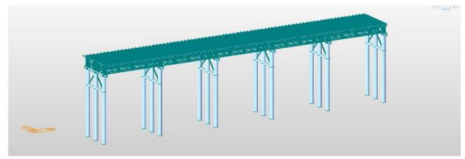
Figure 6-1. Model of trestle finite element
