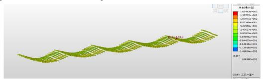
Figure 6-4. Strength check stress diagram of the horizontal distribution of the i-beam (unit: MPa)
