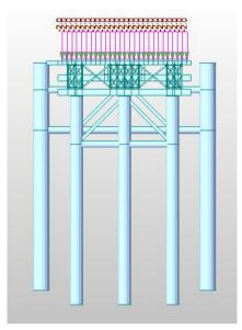
Figure 4-1. Diagram of uniform construction load
