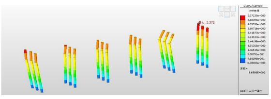
Figure 6-10 Deformation diagram of steel pipe pile (unit: mm)
