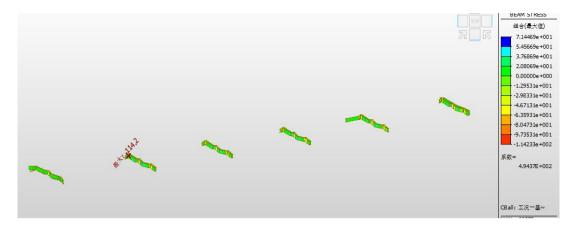
Figure 6-7. Strength check stress diagram of pile beam i-beam (unit: MPa)
