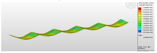
Figure 6-2. Strength check stress diagram of bridge panel (unit: MPa)
