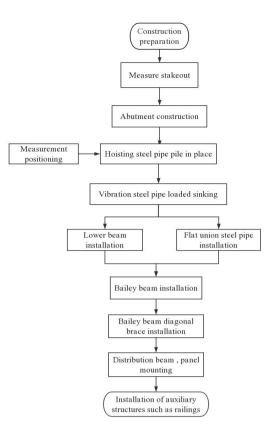
Figure 2-1. Flow chart of the construction process of the trestle
