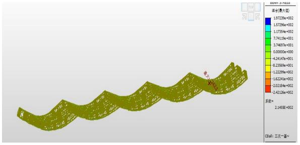
Figure 6-5. Strength check stress diagram of Bailey beam (unit: MPa)
