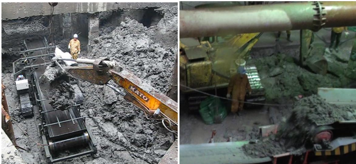
Figure 7. Field tests of the track-type belt conveyor.
