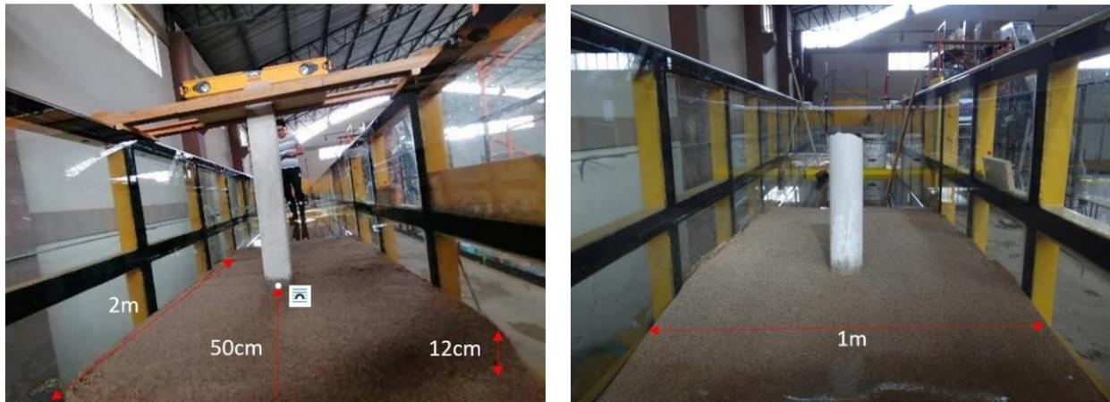
**Figure 1.** Location of the square and circular pile on the sand bed.
