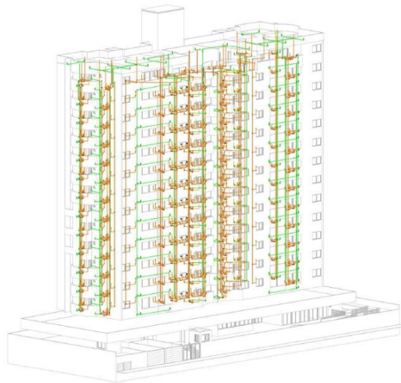
Figure 4. Three-dimensional plumbing model. Source: the authors (2020)
