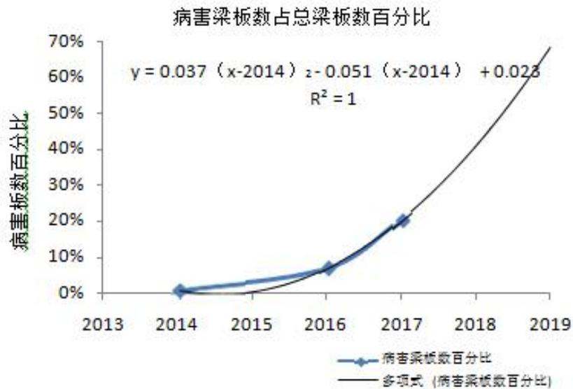
**Figure 4.** Forecast of the growth of down-Line bridge diseases
