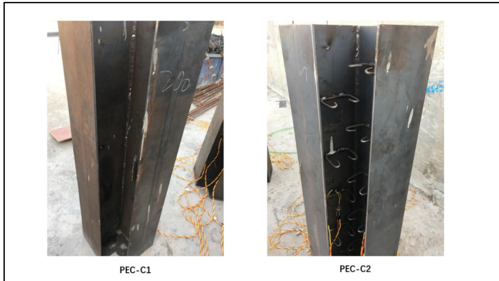
Figure 2. Photos of cross-shaped PEC column PEC-C1 and PEC-C2
