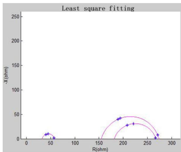
Figure 11. Impedance spectrum trace of human body section.
