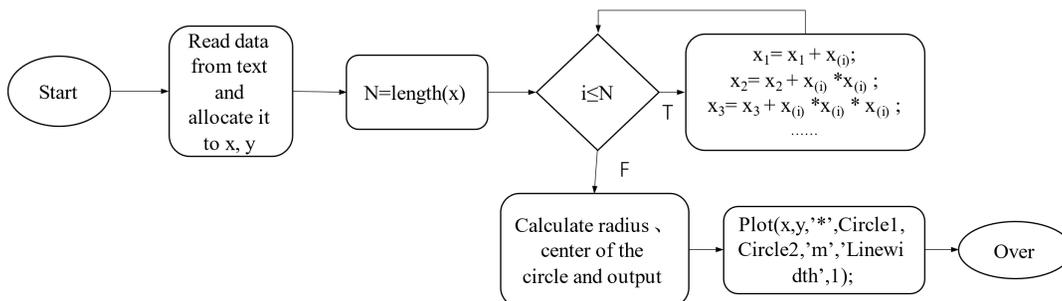
Figure 5. Flow chart of bio-impedance spectrum fitting.
