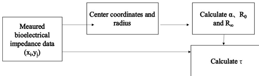
Figure 3. Steps of extracting feature parameters.
