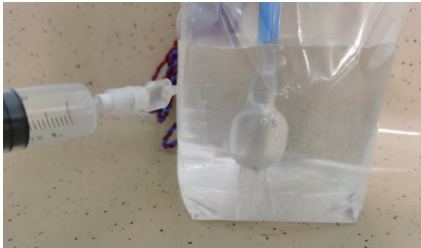
Figure 3. Inflate the ENG ETT with 20ml air by a syringe, through the cuff inflation valve; continuous bubbles emerge from the two cuff splits
