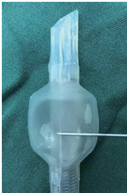
Figure 2. There were two splits on the cuff of the replaced EMG ETT
