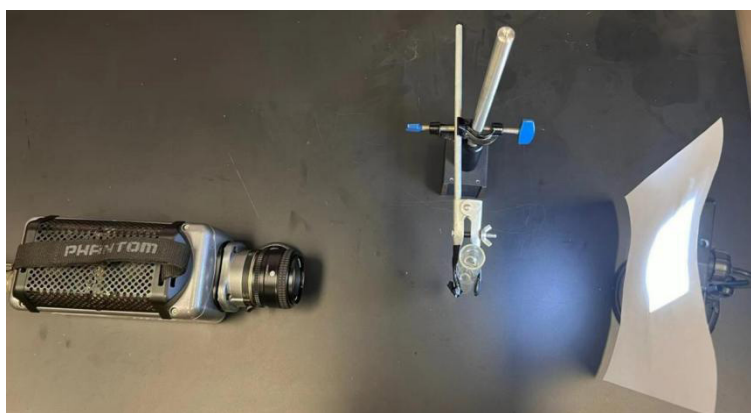
Figure 5. High-speed photography equipment and experimental setup layout
