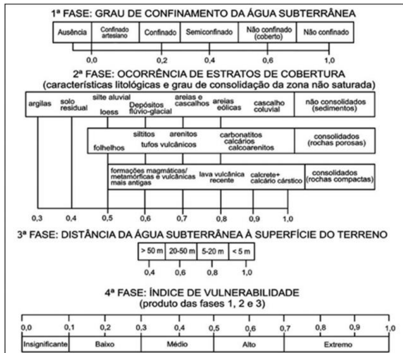
Fig. 2. Stages for determining the vulnerability index using the GOD methodology
