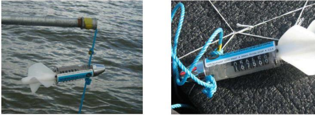
Figure 5. Mechanical flowmeters used to determine velocity
