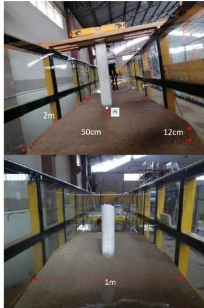
Figure 1. Location of the square and circular pile on the sand bed
