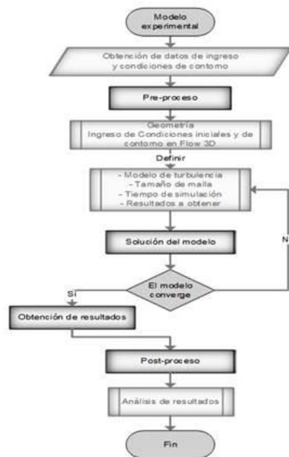
Figure 2. Flowchart of the experimental model
